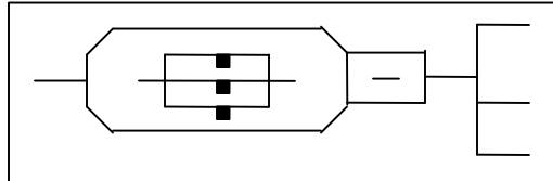
This symbol indicates that all the child elements (shown on the right side of this symbol in a schema diagram) have to be specified, but, they can be specified in any sequence.
